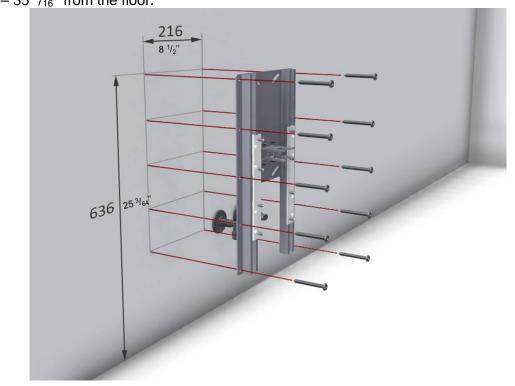
The measurements on the wall, shown below, enable the wash basin to be height adjusted 29  $^{17}/_{32}$  "- 35  $^{7}/_{16}$ " from the floor.
