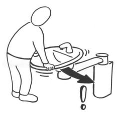
Ropox Swing Wash Basin has a turning function, which means that it is <u>NOT</u> allowed to be used as a walking or standing support.
