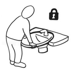
If the wash basin is locked in the Dock-in it functions as a standard wash basin and is safe to use as a standing support.
