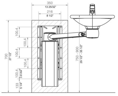
always consider the material, condition and strength of the wall and use screws and rawlplugs suitable for the specific wall type.
