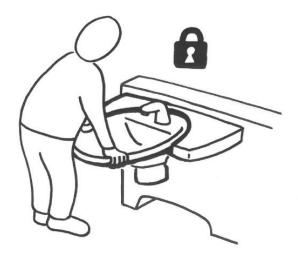
Ropox Swing Washbasin has a turning function, which means that it is <u>NOT</u> allowed to be used as a walking or standing support.
