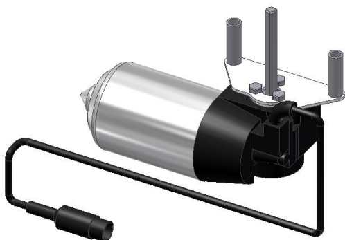
6.6.1 Motor, with spindle, is mounted through back plate and into gearbox
