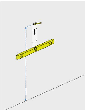
Mark the holes in the mounting template based on the desired height.
