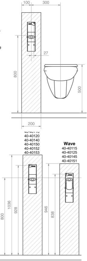
Attached is the mounting template with an indication of the 6 mounting holes on the bracket. User heights (upper edge of toilet support) and installation heights (upper holes in template / bracket)
