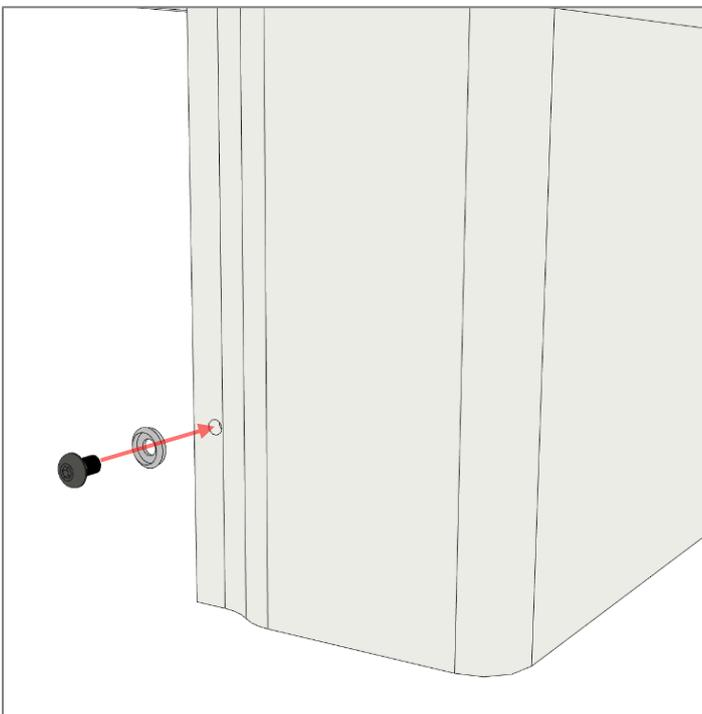
When all the wires have been attached and screws fastened, the cover must be fixed in place. Use the attached M5x8 screws and screw button cover. This step can wait until the end to make it easier to access the control box and wires if needed.
