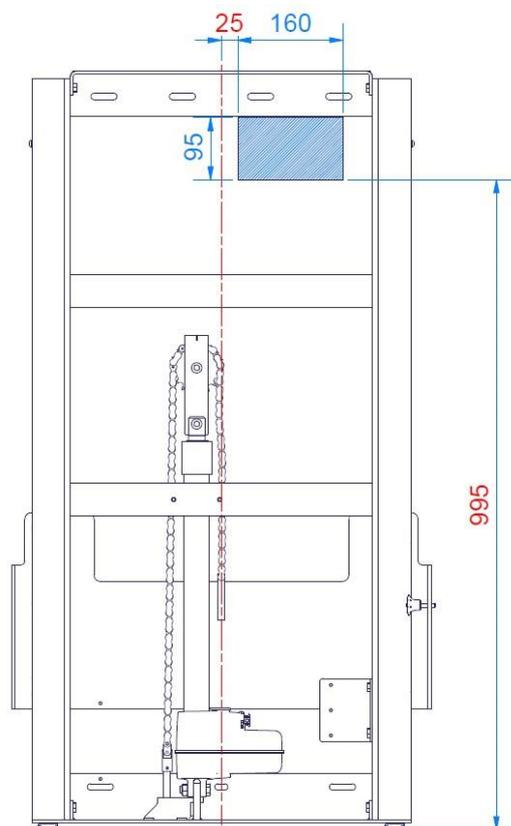
The following drawing illustrates the space that can be allocated for an electrical outlet without interfering with the movement of the unit. The blue-hatched area is the safe area for placing an electrical outlet and cover. Placing the outlet and/or cover outside of this area may result in product damage and malfunction.
