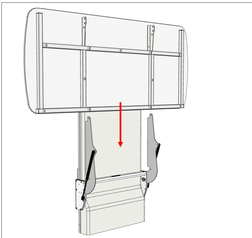
Slide the tabletop in between the lifting unit and the support arms on the lifting unit. It is an advantage to be two persons when doing this.
