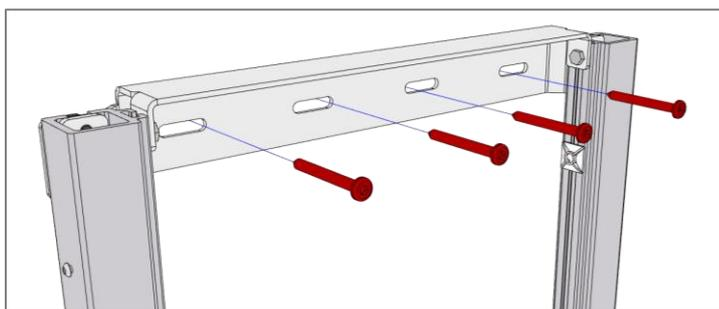
**Maximum pull force for each of the four screws in top of the unit: 40kg**
