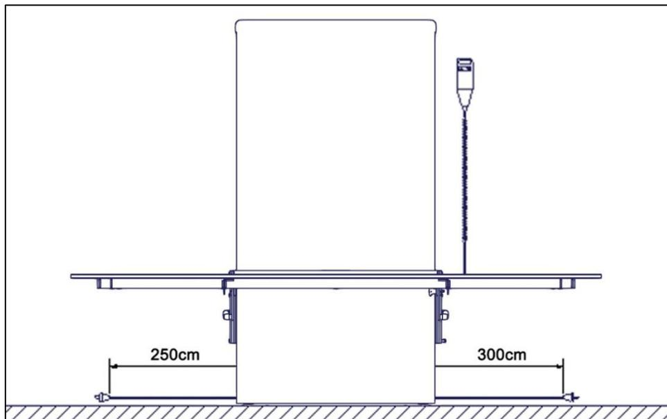
The main power cable has a total length of approx. 320cm of which 250cm is outside the lifting unit. The cable can be pulled out in either left or right side.
