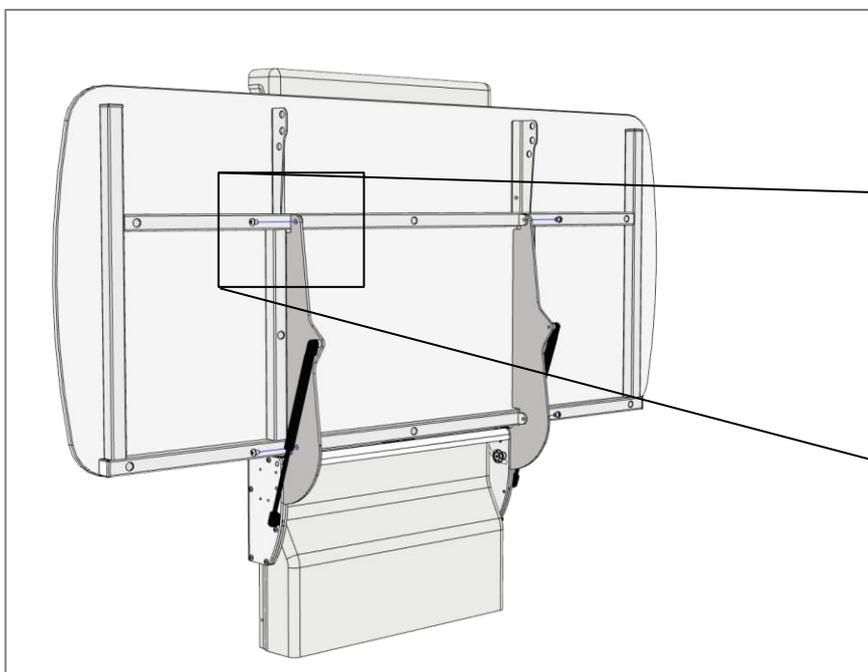
Fasten the tabletop to the Lifting unit with 4 pcs. M8x12 through the bushings in the support arms.
