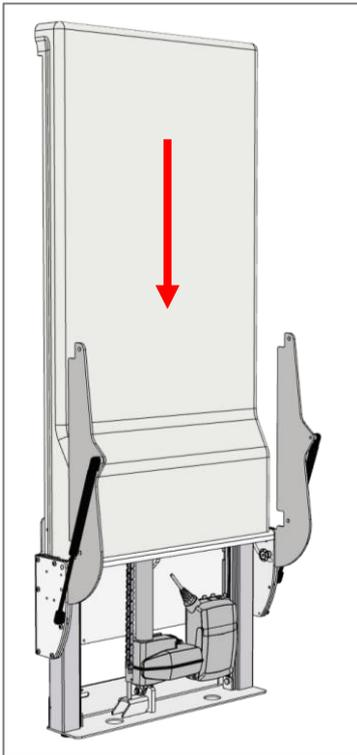
The cover can either be clicked in place from the front or slide down from above. Make sure that the cover reaches the floor and is in contact with the wall at the top. This step can also wait until the end of the installation process if ease of access to the electrical components is required.
