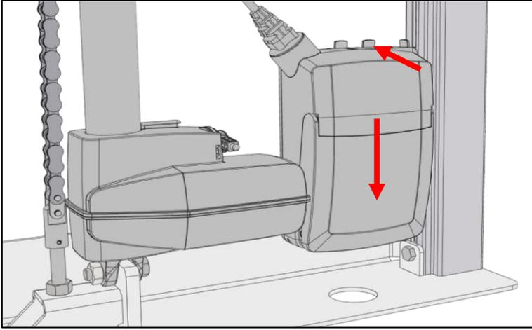
To gain access to all the bottom holes, the control box will need to be temporarily removed. This is done by unlocking it from the holder at the top, pressing it back and sliding the control box down.
